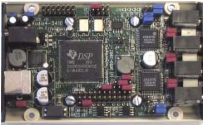
FIGURE 1.1. Audio4-5410 board - LINE IN configuration
