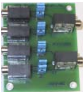
FIGURE 1.4. Quad microphone adaptor
